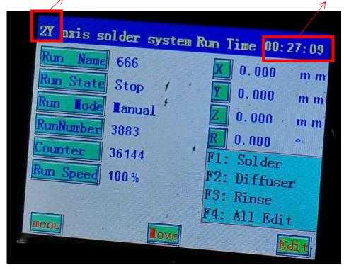
Cycle time:=27s(include loading&unloading time)
